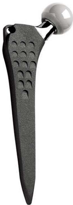
Fig. 1. The titanium alloy (titanium, 6% aluminum, 4% vanadium) implant used in this study features a tapered wedge geometry, rectangular in cross-section, with a sand-blasted surface (C2 stem; Lima Corporate S.P.A, Udine, Italy).
